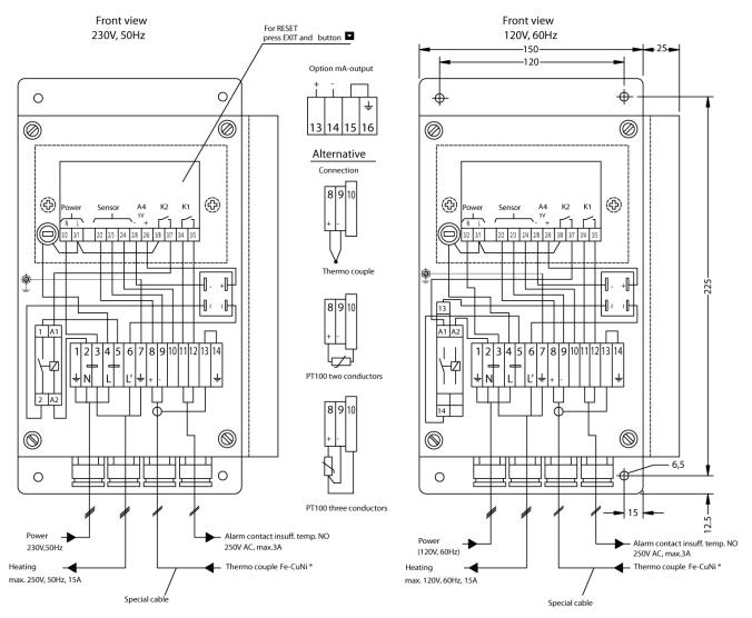
Figure 3 Electrical wiring plan
