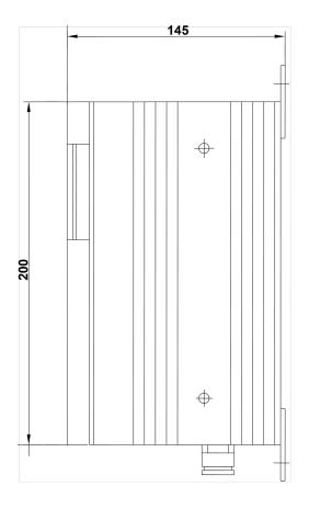
Figure 2 Housing dimensions and installation dimensions
